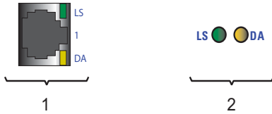
Figure 9: Port status LEDs 1 – Port status LEDs for RJ45 2 – Port status LEDs for DSC
