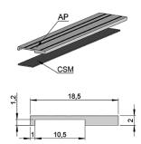
Stainless steel cover for protection. To be placed in the magnetic band (10 mm width - 0.3 mm thickness).
