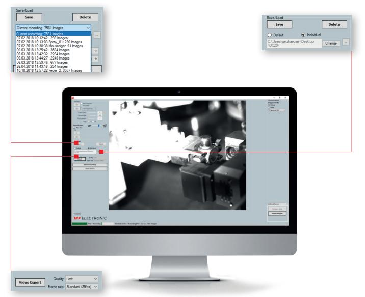
The **video export** creates a file in avi format that is suitable for sending via email or that can be used for documenting the recordings. All additional information relevant to the recording (e.g., time stamp, signals from sensors) are also permanently stored when saving and exporting the video.
