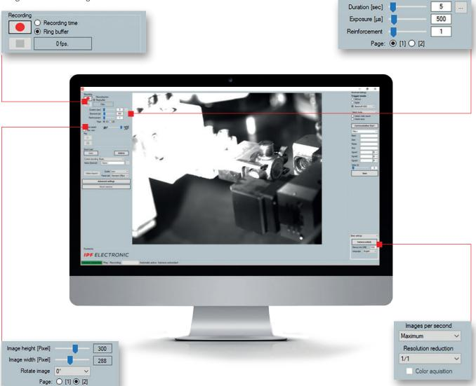
**Image height** and **width** can be set flexibly to optimize the image cropping and the achievable frame rates. The **rotate image** option (rotate the camera images in increments of 90°) also ensures maximum flexibility during camera installation on-site.
