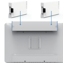
Battery module contains 2 x battery packs
