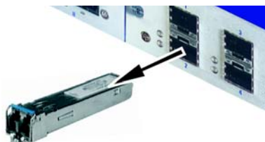
Figure 8: Deinstalling an SFP module
