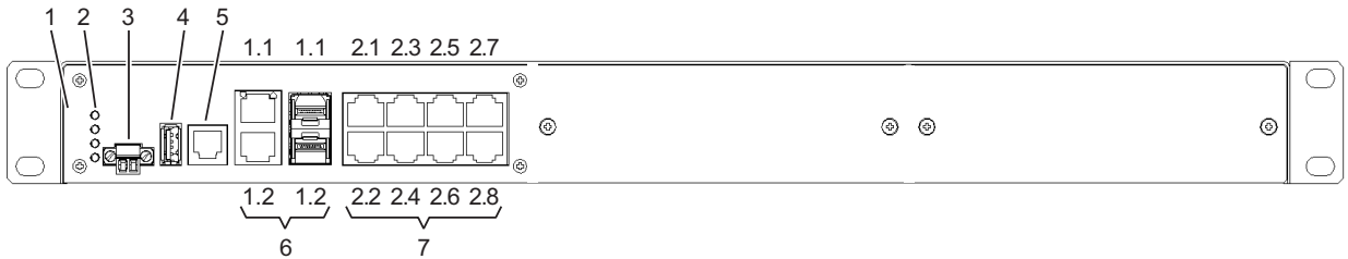
Figure 2: Overview of interfaces and display and control elements in the MACH 102-8TP-F and MACH 102-8TP-FR
