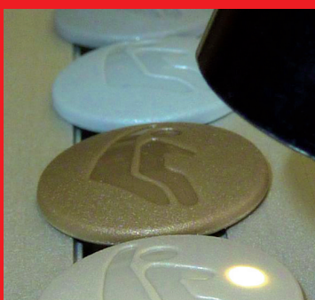
▲ Color inspection of control elements in car interiors
