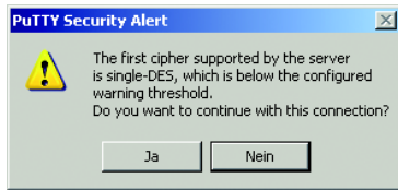
Figure 80: Security query at the defined warning threshold
