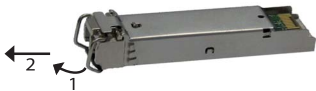
Figure 10: Deinstalling an SFP transceiver
