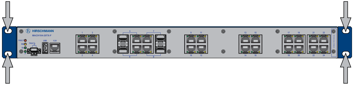
Figure 14: Mounting the MACH104 in the 19" cabinet
