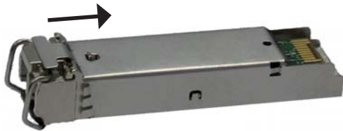
Figure 11: F/O SFP transceiver
